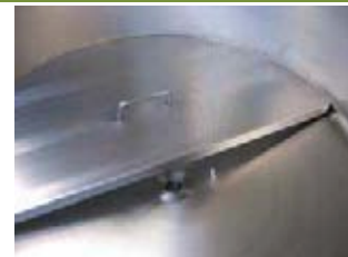
Lauter tank - two part perforated plate
