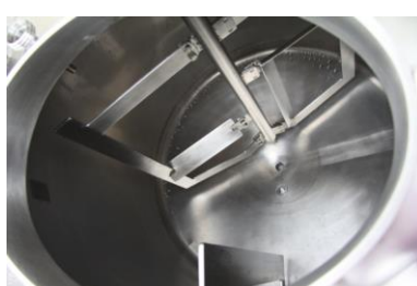
Anchor (gate) stirrer with stirring barrier (100mm from the wall)
