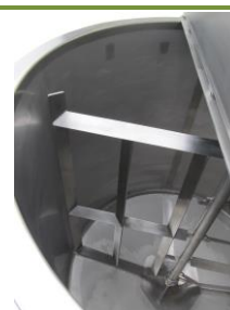
Anchor (gate) stirrer near the wall (10-15mm from the wall)
